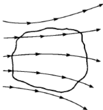
Finite control volume fixed in space with the fluid moving through it.
